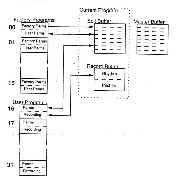
The Cyclone leaves the factory with 32 Programs: 00 through 15 are Factory Programs, while 16 through 31 are User Programs (an optional memory upgrade adds 68 more User Programs for a total of 100 Programs). The two types of Programs are described as follows:
